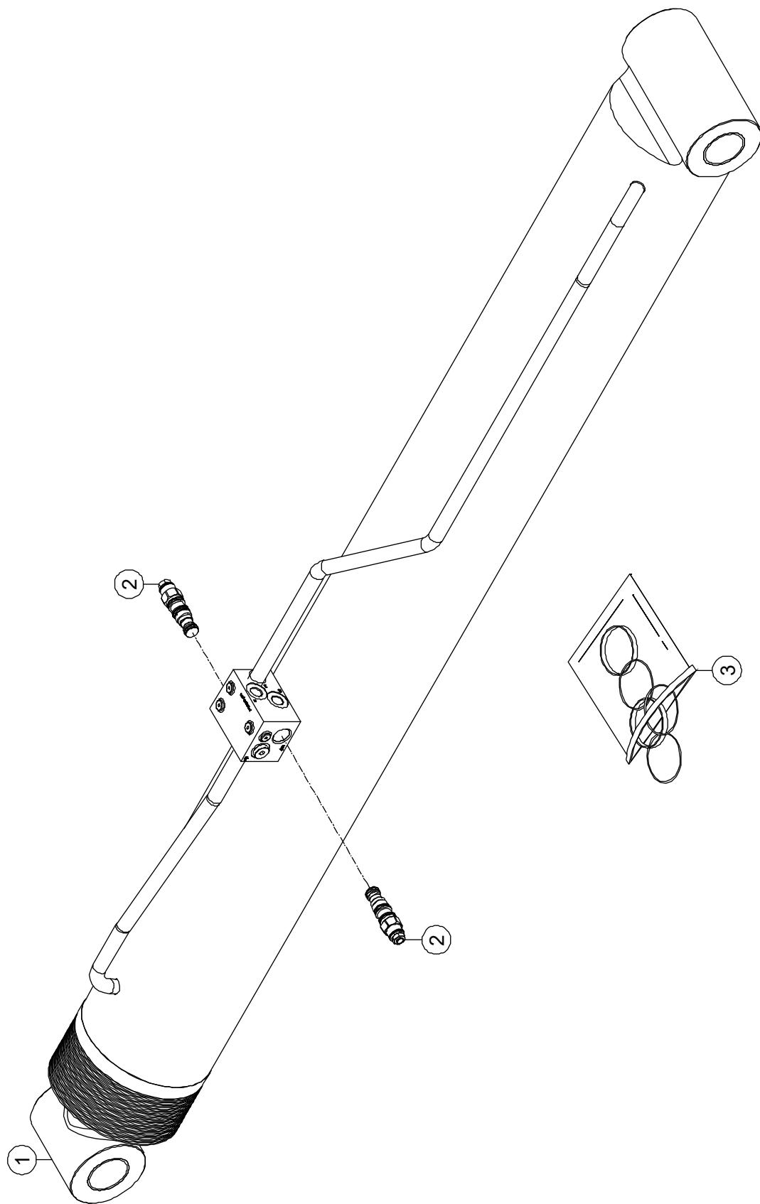
**5-4 Lifting Cylinder Assembly (BT20CRT2, BT18CRT2, BT16CRT2)**
