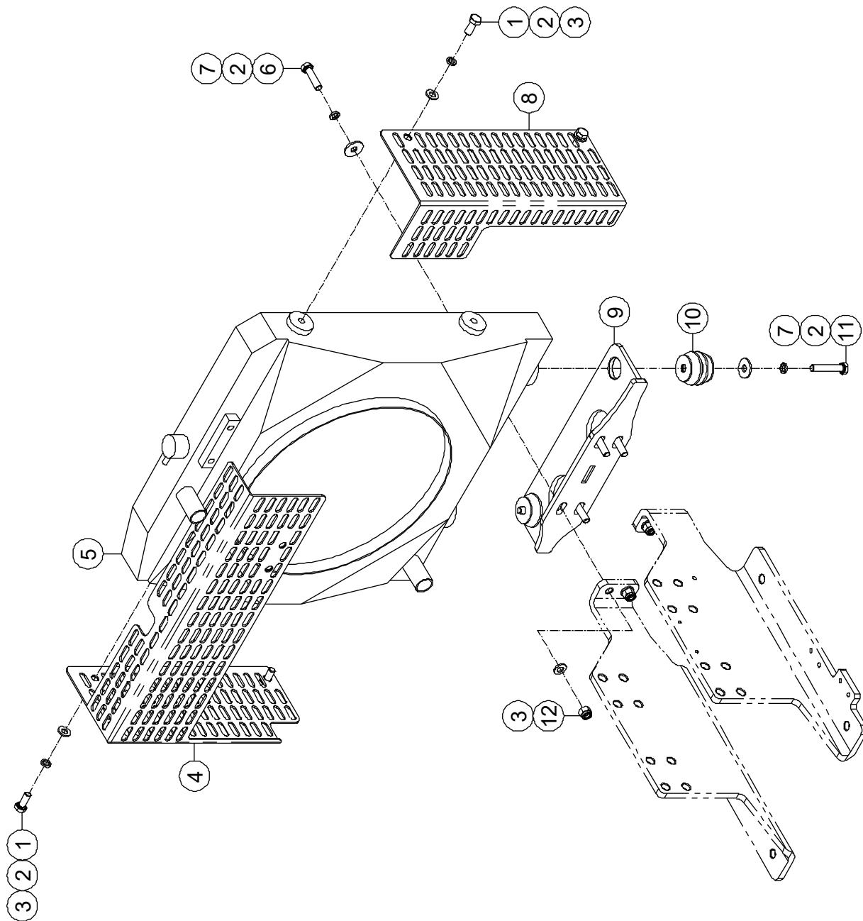
**1-17 Engine Cooling System Installations 1 (Perkins Engine)**
