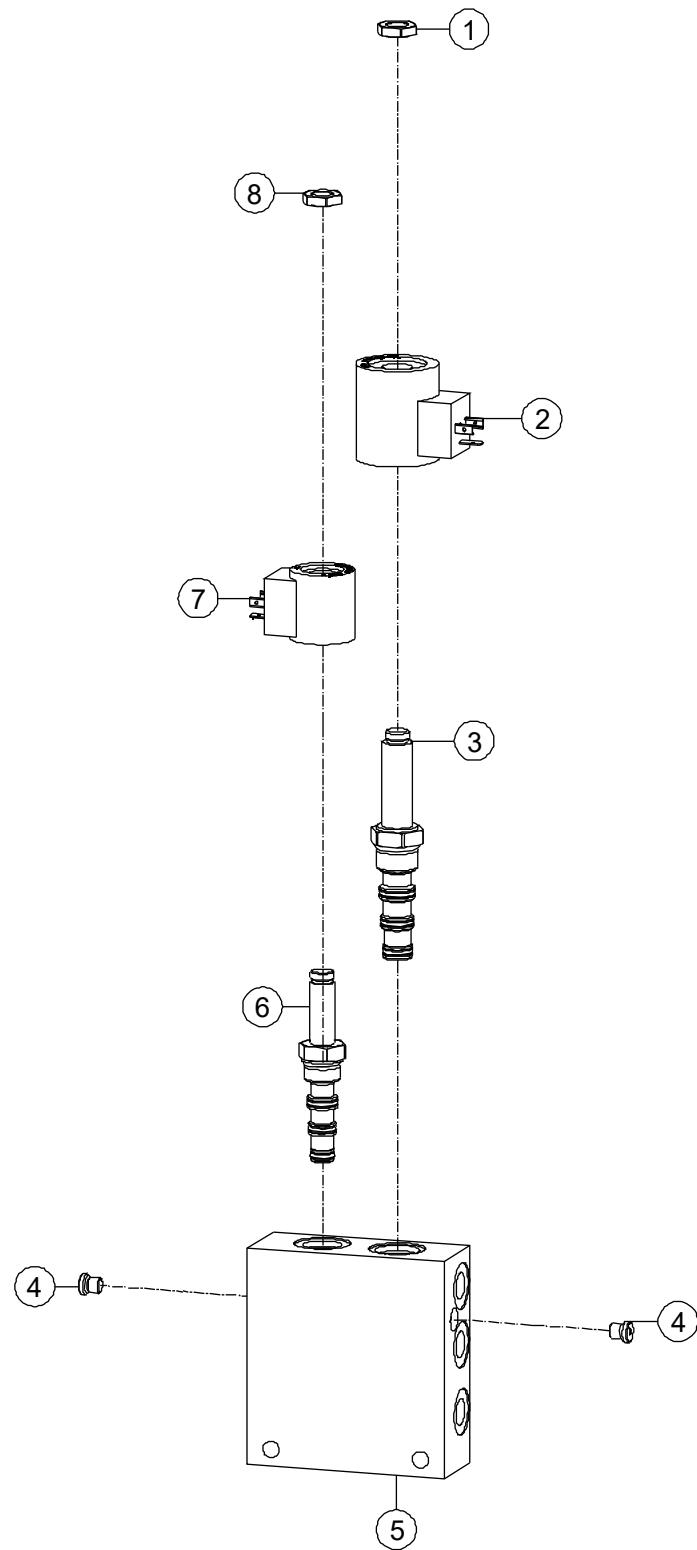
**Figure3-30 Directional Valve Assembly**
