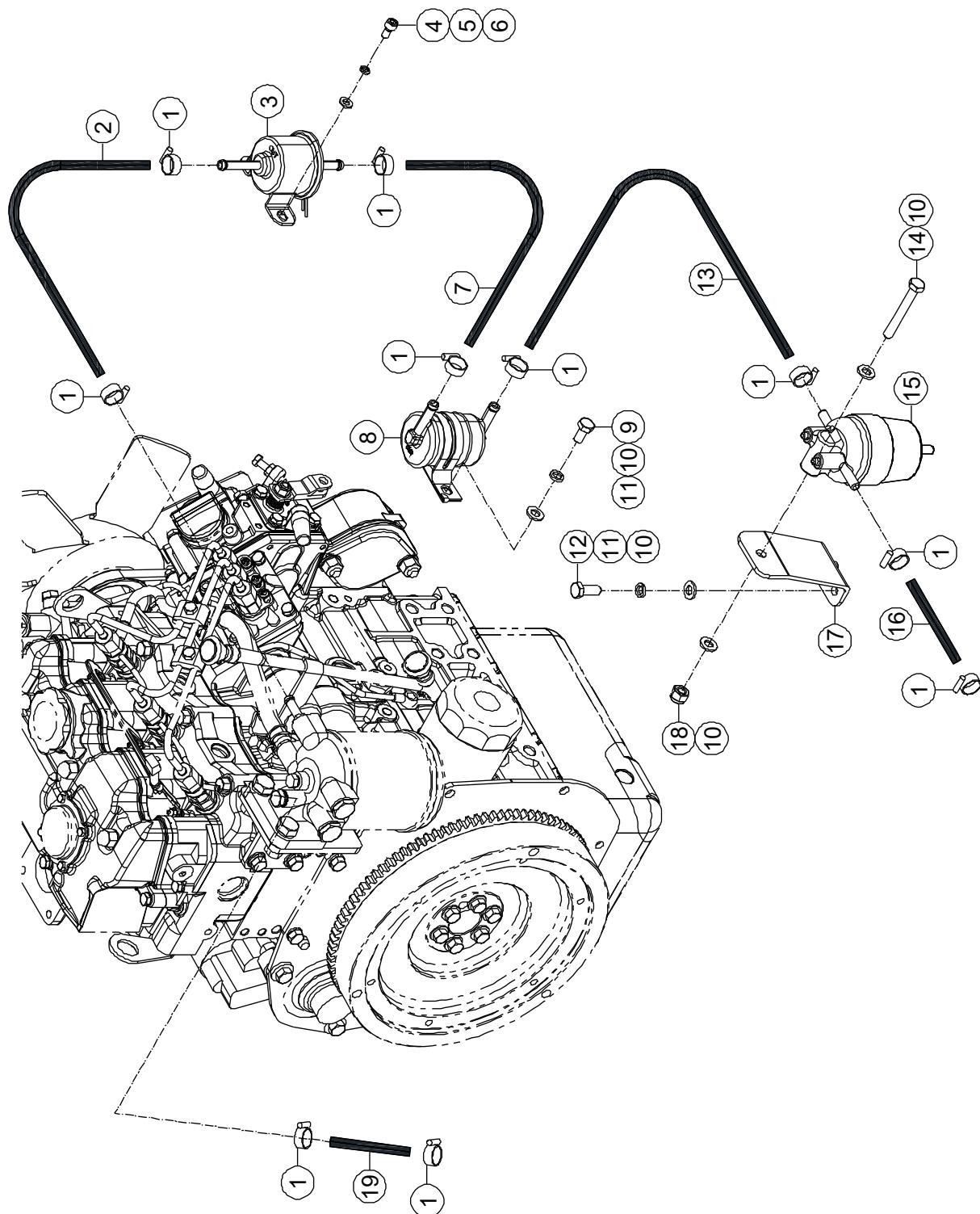
**1-25 Engine Fuel System Installations (Perkins Engine)**
