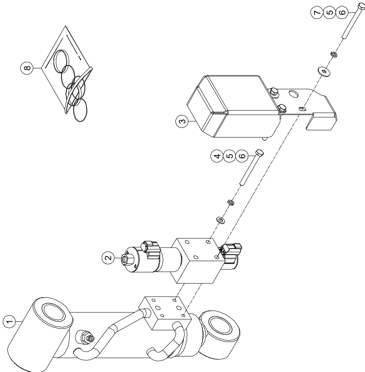
**5-1 Left Axle Lockout Cylinder Assembly**
