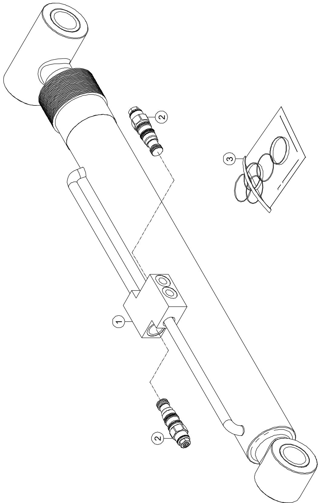
**5-8 JIB Lifting Cylinder Assembly**
