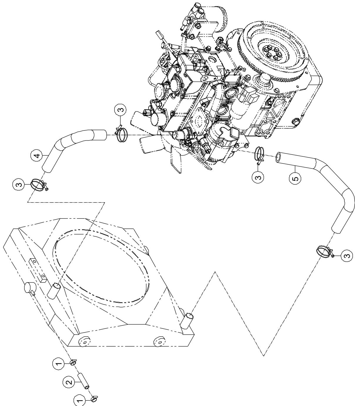
**1-19 Engine Cooling System Installations 2 (Perkins Engine)**
