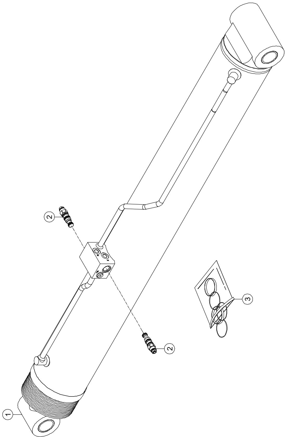
**5-3 Lifting Cylinder Assembly (BT22CRT2)**
