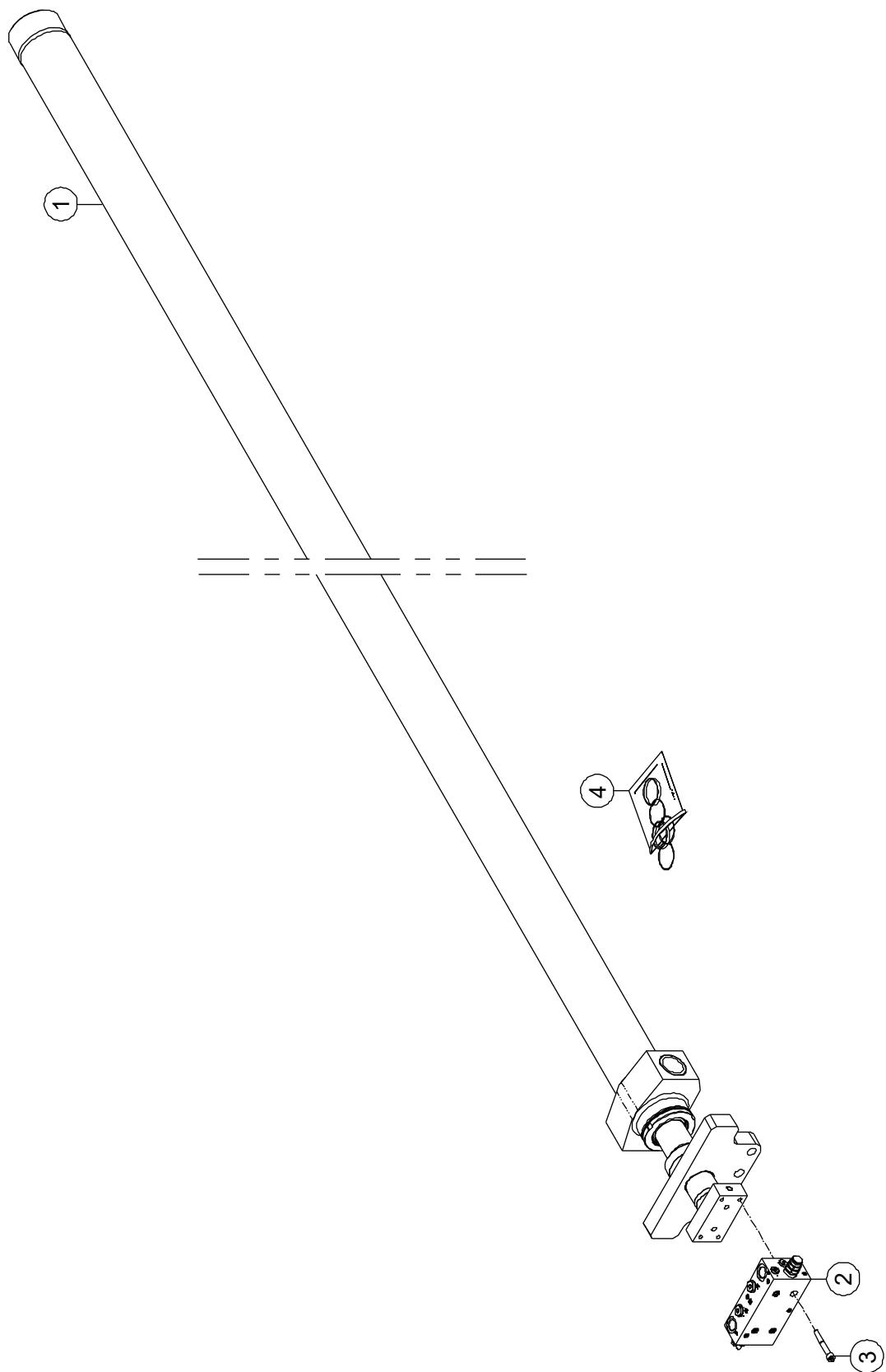
**5-5 Telescope Cylinder Assembly (BT22CRT2)**
