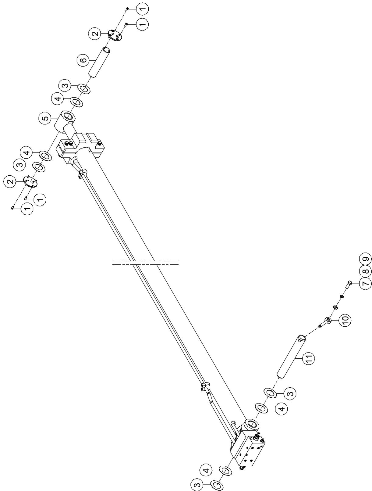
**3-19 Telescope Cylinder Assembly Installations (BT20CRT2,
