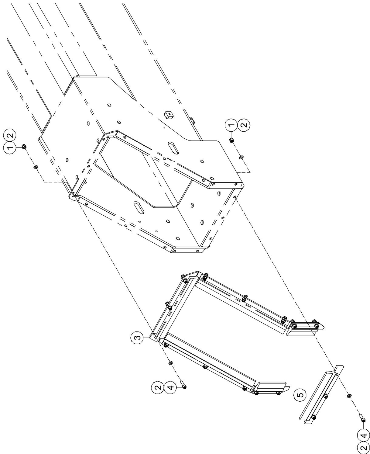
**3-24 Boom Shield Installations (BT20CRT2, BT18CRT2, BT16CRT2)**
