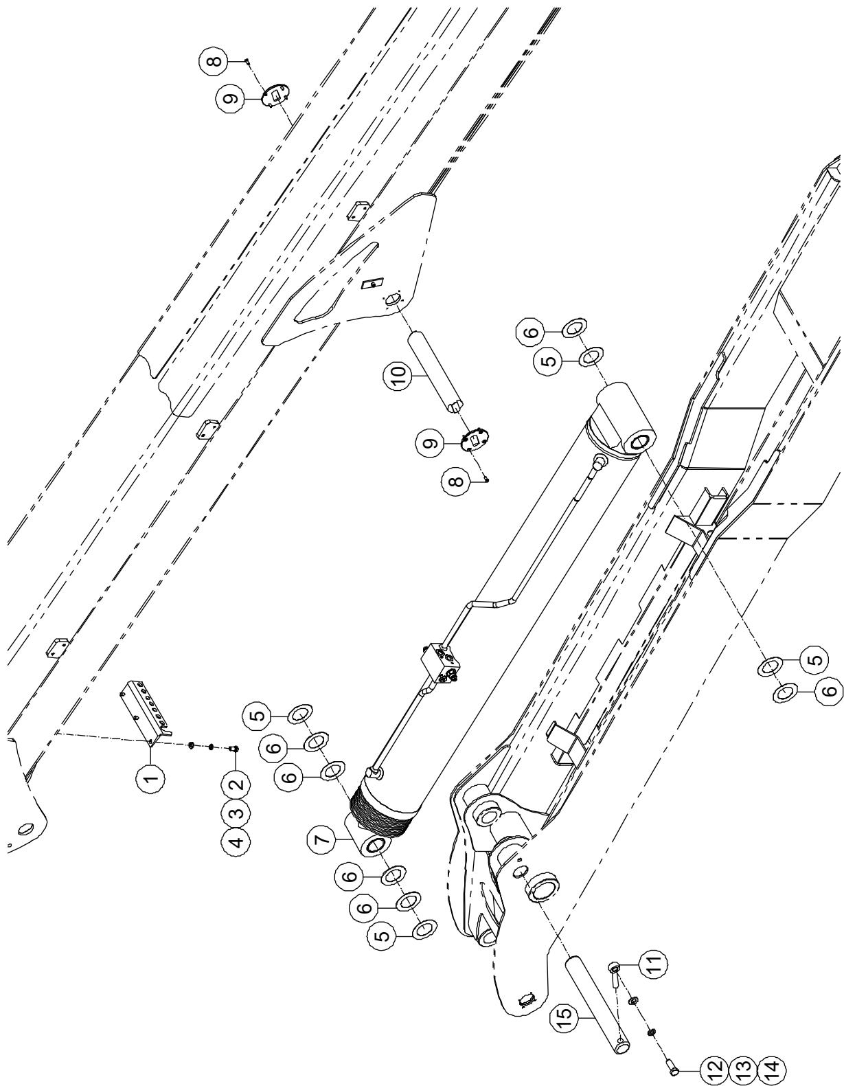
**3-4 Lifting Cylinder Assembly and Boom Installations (BT22CRT2)**
