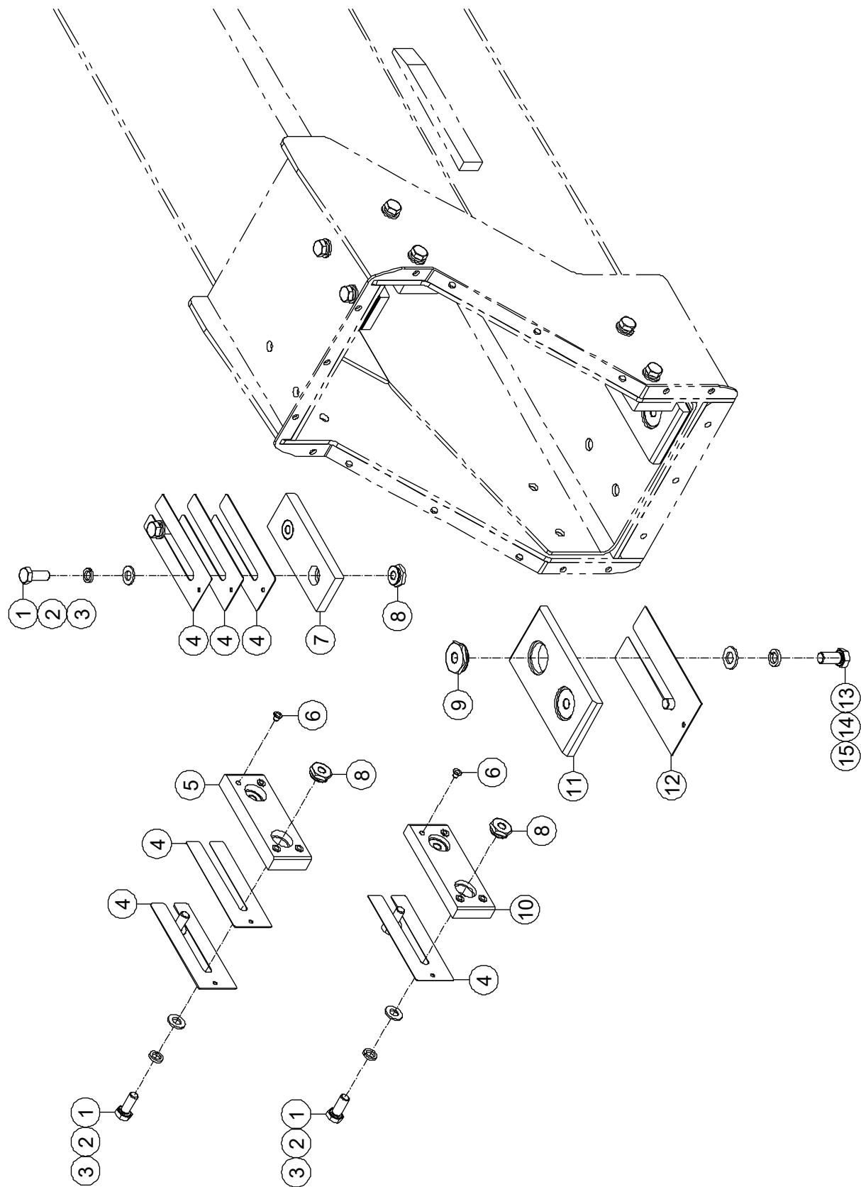
**3-13 Second Boom Sliding Block Installations 1 (BT22CRT2)**
