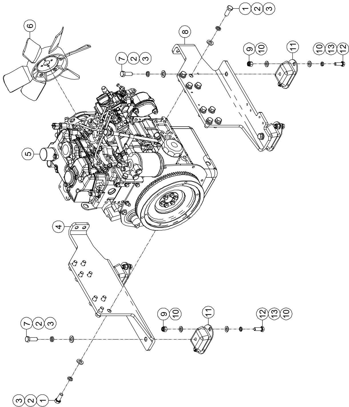
**1-15 Engine Assembly (Perkins Engine)**
